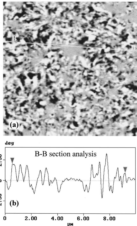
FIG. 3. Magnetic-force image with a scan size  $10 \times 10 \mu\text{m}$  for the  $\text{Nd}_{60}\text{Al}_{10}\text{Fe}_{20}\text{Co}_{10}$  BMG annealed at 715 K for 1.8 ks (a), and typical section-analysis result (b).
