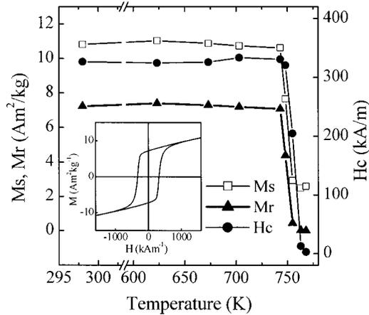
FIG. 1. Dependence of  $H_c$ ,  $M_s$ , and  $M_r$  on isothermal annealing temperature for  $\text{Nd}_{60}\text{Al}_{10}\text{Fe}_{20}\text{Co}_{10}$  alloy (annealing for 1.8 ks). The inset shows the hysteresis loop at room temperature.
