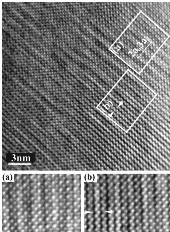
FIG. 2. The [0 0 1] zone-axis HREM image of CR-0 sample obtained at 93 K.
