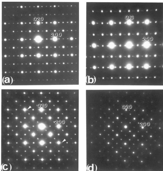
FIG. 1. Selected area diffraction patterns recorded from samples CR-0, CR-1, CR-3, CR-5, all recorded at 93 K.
